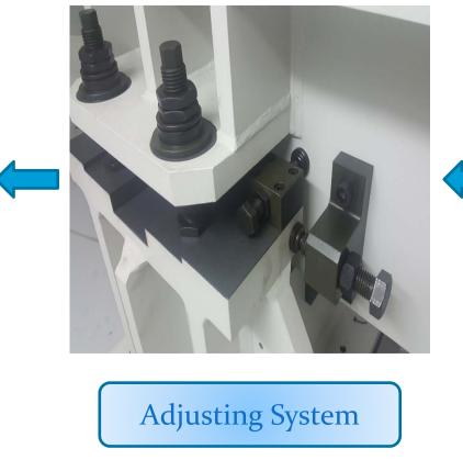
Horizontal and Vertical Wedges /Girder -Girder Alignment 3 Pint Contact During Alignment Vertical Adjusting System
