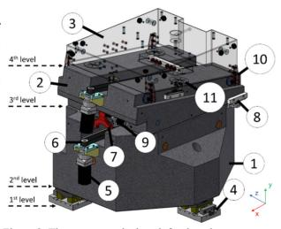
under the terms of the CC BY 3.0 licence (© 2018). Any distribution Figure 2: Three-part granite bench for the mirrors systems: (1) bottom granite; (2) middle granite; (3) top granite (transparent for visibility); (4) wedge-leveller; (5) stepper motor for Tx; (6) timing belt for Tx; (7) commercial airbearing guiding for Tx; (8) optical encoder; (9) power screw mechanism for Ry; (10) commercial air-bearing for wedge; and (11) machined air-bearing pad.
