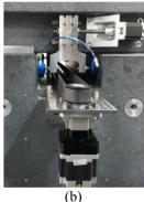
Figure 3: (a) 4CM granite bench assembled at the hall of the metrology building of LNLS; (b) Detail of Tx and Ry stepper-driven actuation mechanisms with the timing belt and power screw, guided by the commercial air pad.
