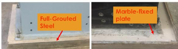
Figure 7: Prototypes with full grouted bottom surface.
