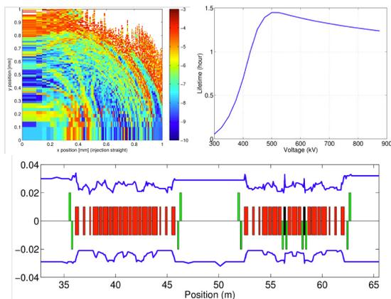
Figure 3: (Top Left) Frequency map for the 9BA lattice. (Bottom) Local momentum aperture for two periods including Superbends. (Top Right) Touschek lifetime as a function of RF voltage. All calculations include lattice errors and physical apertures.
