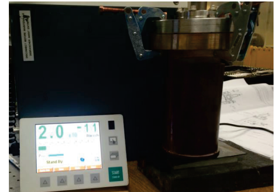
Vacuum Leak Test
