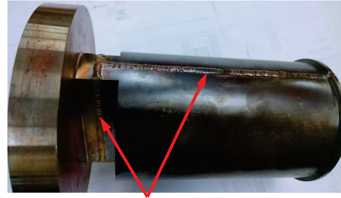
Full Penetration Welds in a Prototype
