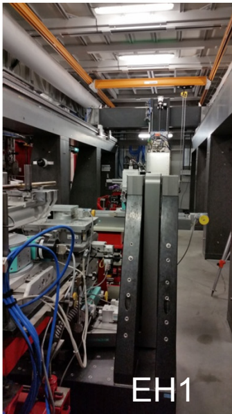
Laue-Laue monochromator At 105m from the source
