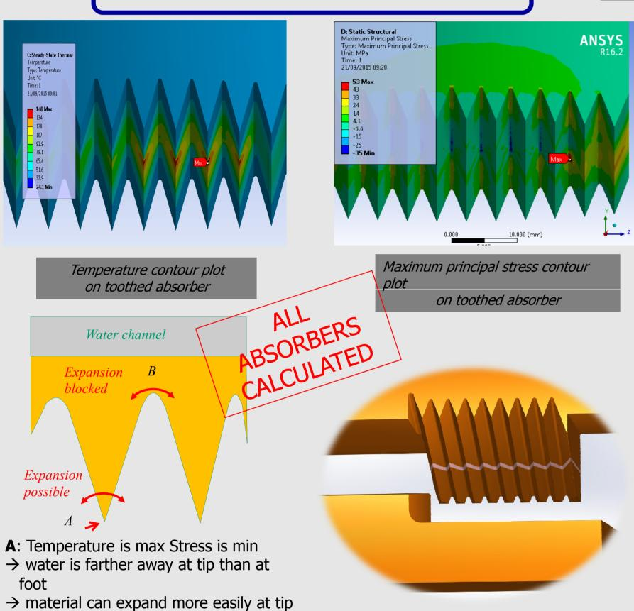
than at foot B: Temperature is min Stress is max  $\rightarrow$  water is closer at foot than at tip  $\rightarrow$  material cannot expand easily at foot
