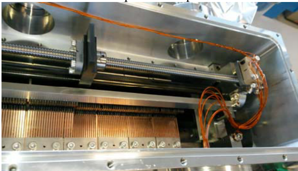
Figure 1: A general view of the F-Switch from above. The leadscrew and claw actuator shaft are visible along with a number of the bistable springs. The lenses are all hidden below this view.
