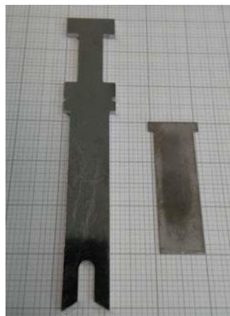
Figure 5: An actuator blade alongside a fixed spacer. Wire EDM was found to be the most cost-effective method of production for these parts. These examples are not yet DLC coated.
