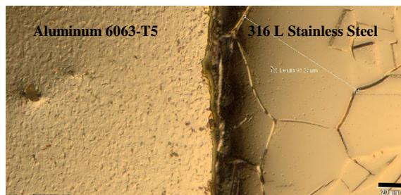
Figure 10: Friction weld of aluminum to stainless.
