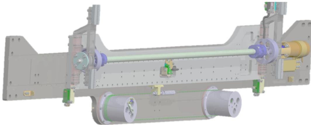
Figure 12: Beamstop actuator.
