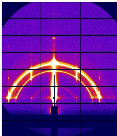
Figure 11: GISAXS image showing beam stop shadows.
