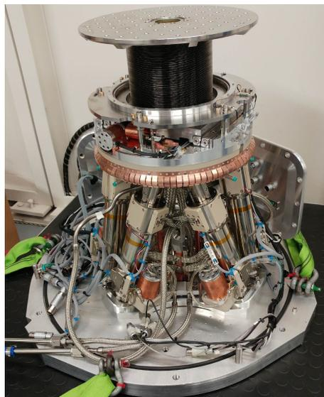
Figure 4: GISAXS Manipulator Stack.
