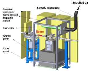
Figure 1: Schematic 3-D drawing of secondary source slits.
