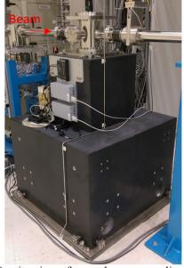
Figure 2: On-site view of secondary source slits installed in the Coherent X-ray Scattering beamline at TPS.
