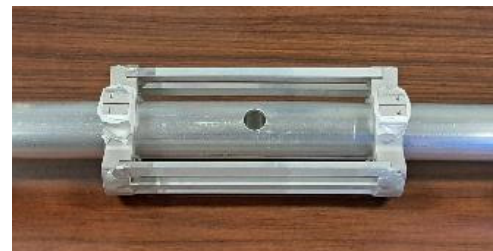
Figure 1: EP tool with the cavity B9AS-AES-003 (top). Patented cathode structure used for EP the cavity (bottom).
