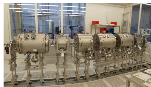
Figure 2: Fully assembled cold string on rail system.
