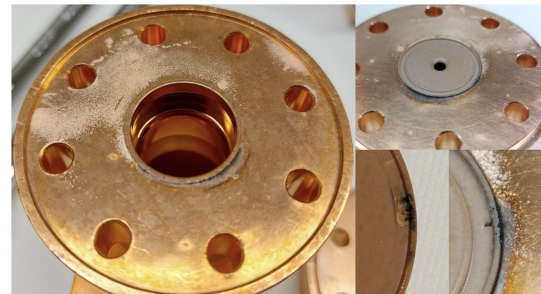
Figure 1: Damage seen on the copper and ceramics from the single cell DDA high power experiment.
