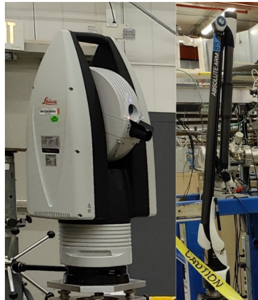
Figure 1: Leica AT960 (left) and Hexagon Absolute ARM 85 (right).
