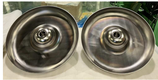
Figure 7: Fabricated lid sections (left: "a", right: "b").
