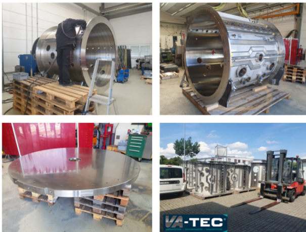
Figure 2: Production of cavity sections and end plates at VA-TEC, Germany.
