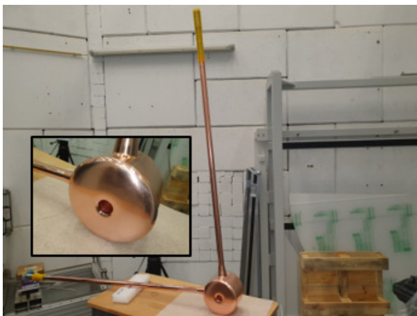
Figure 5: Drift tube and two stems after copper plating at an external galvanic work shop (GALVANO-T, Germany).
