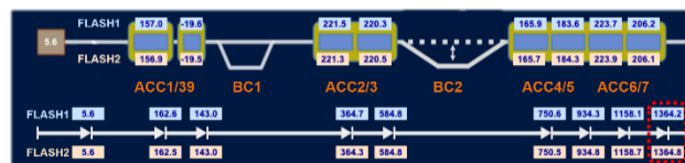
Figure 8: Energy profile along the accelerator calculated from monitoring system. (All values shown are in MeV).
