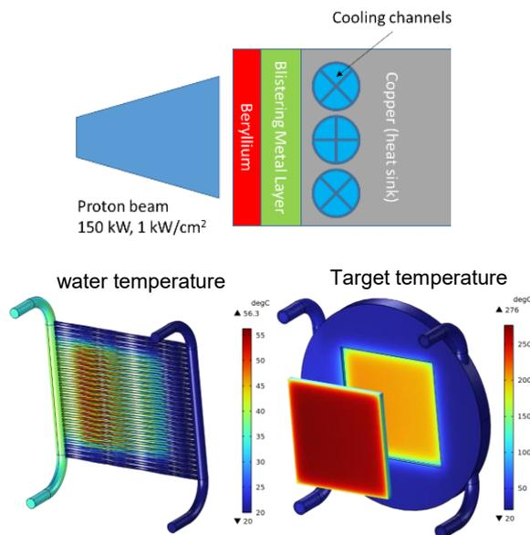
Figure 7: Three-layer target concept and thermal simulations with visible the microchannel cooling system.
