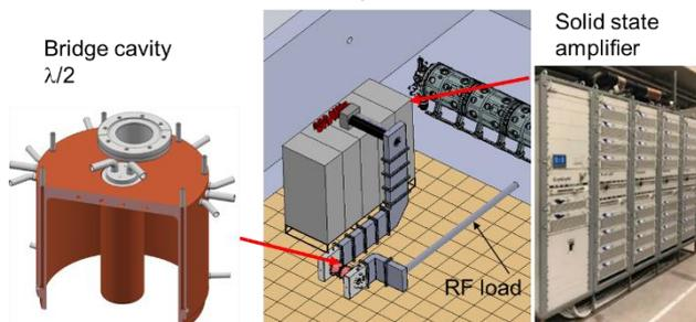
Figure 5: RF tests at LNL (scheme and main elements).
