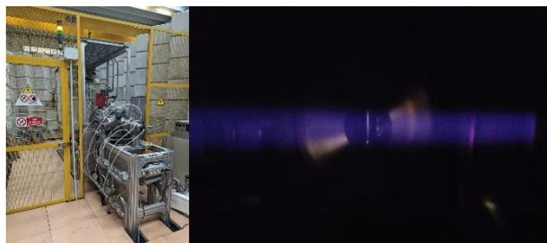
Figure 4: On the left the proton source assembly. On the right, snapshot of the 30 mA 80 keV beam from the ion source.
