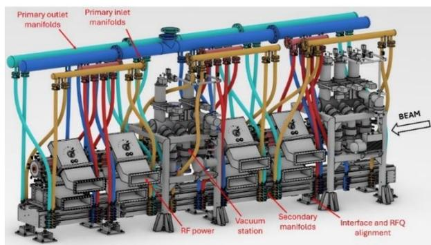
Figure 1: The RFQ integration on the new support.
