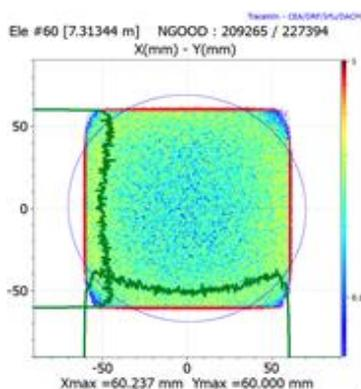
Figure 6: beam spot at the target obtained with proper setting of quadrupoles, octupoles and collimator.
