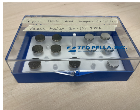
Figure 4: Picture of sample storage box: Samples on the left side of the box were collected from the gun section of the e-Linac and have been coated in carbon for SEM analysis. Samples on the right show pre-mounted stubs with covers still in place as they were not used for collection.
