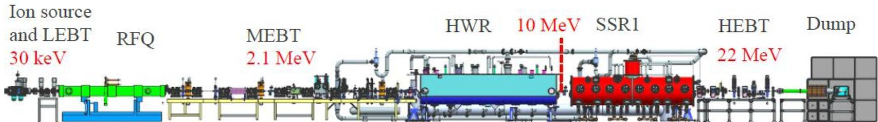
*LEBT = Low Energy Beam Transport; RFQ= Radio Frequency Quadrupole; MEBT= Medium Energy Beam Transport; HWR = Half-Wave Resonator; SSR1=Single Spoke Resonator; HEBT = High Energy Beam Transport*
