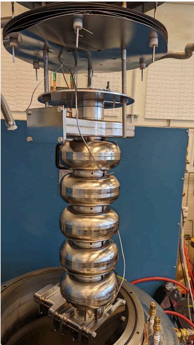
C75 cavity made from large grain Nb. Nicole Verboncoeur | LINAC 2022
