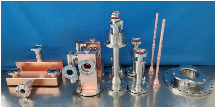
Fig. Fabricated sub-assemblies of 3.9 GHz FPCs
