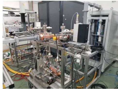
Fig. Test bench for 3.9 GHz FPCs
