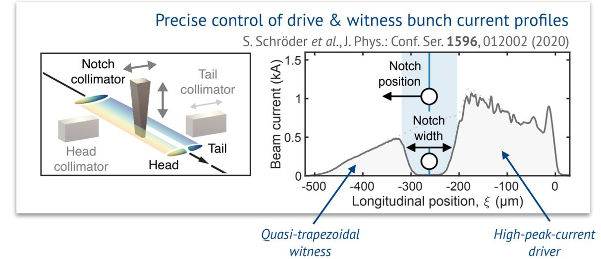
Measurement of optimal beam-loading, demonstrating energy-spread preservation
