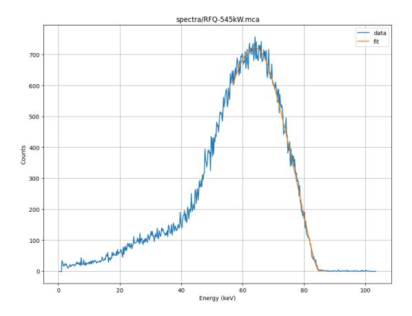
545 kW for full field level confirmed by X-ray measurements.
