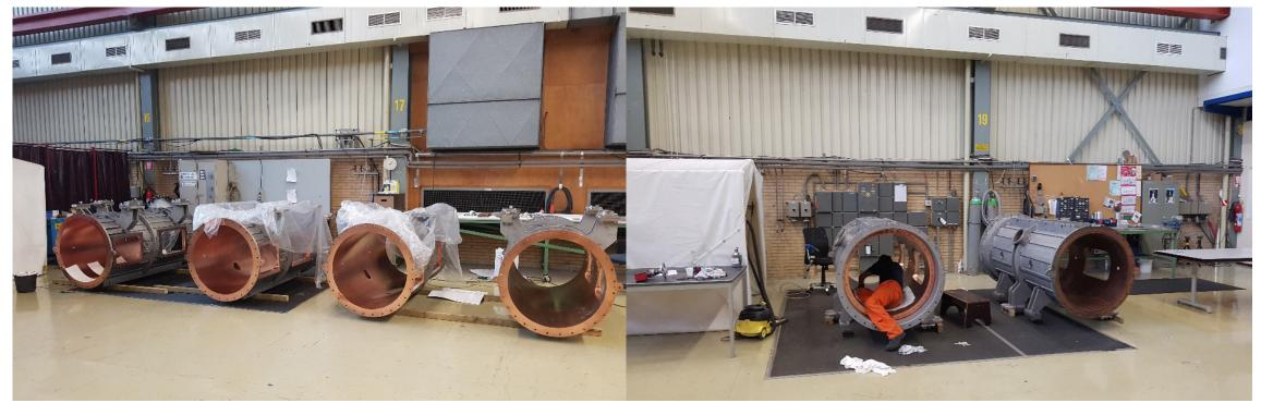
Sections of tank are bolted together with HELICOFLEX<sup>™</sup> seals for vacuum and RF. Could be dismantled in future if necessary.
