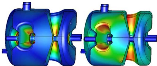
electric field (left) and magnetic field (right)
