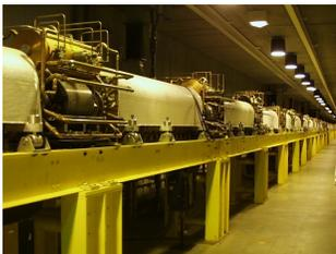
Accelerating tanks of 805 MHz Coupled Cavity Linac
