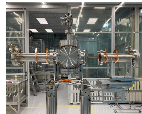
COUPLER ASSEMBLY TO RF CHAMBER
