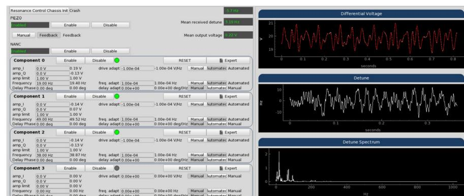
**Up to 4 different microphonics frequencies** can be compensated using totally independent NANC components.
