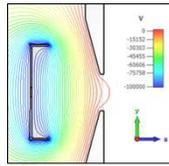
Equipotential lines generated due to the applied potential of -100 kV on cathode
