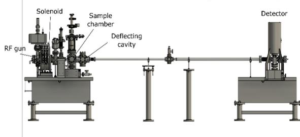
Figure 1: MUED beamline schematic.
