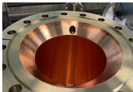
Figure 5: Plating oxidation on vacuum outer conductor.
