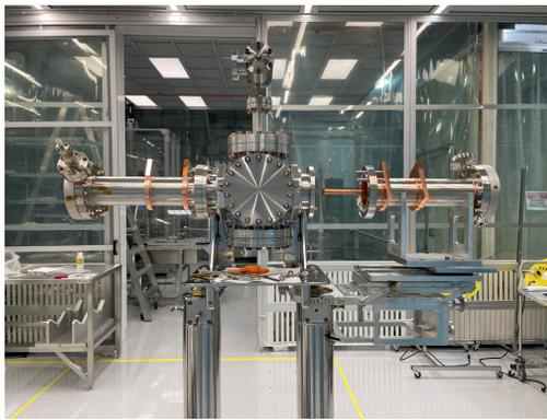
Figure 6: Coupler assembly to RF test chamber.
