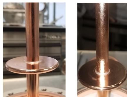
Figure 4: Antenna braze quality and striations. Left: normal lighting, Right: with flash.
