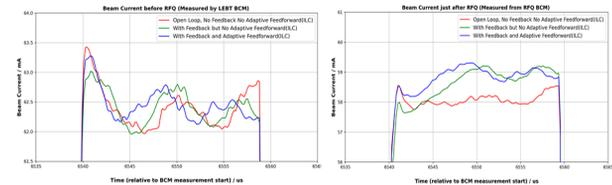
Figure 6: Beam current before (left) and after (right) RFQ under different beam loading compensation methods.
