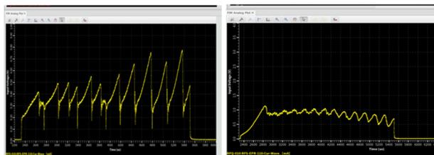
Figure 1: Multipacting patterns vary with RF power level. (Left: electron pickup read at 110 kW, Right: electron pickup read at 80 kW).
