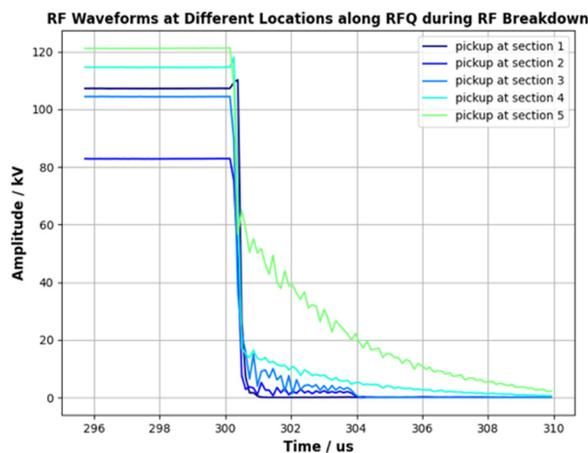
Figure 2: Cavity field measured by pickups located in different sections of RFQ during RF breakdown.
