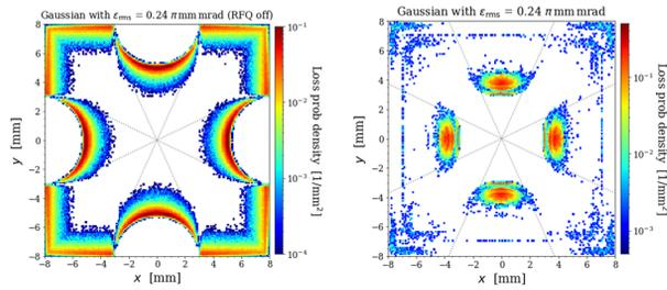
Figure 4: Beam loss distribution simulation in RFQ (left: RF off, right: RF on).
