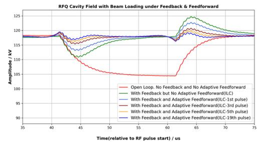
Figure 5: Beam loading compensation by feedback and adaptive feedforward.
