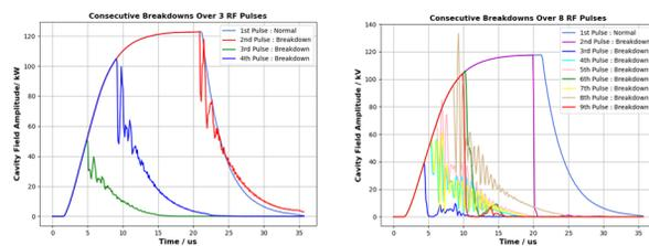
Figure 3: Normal breakdown scenario (left) in which RF goes back to stable after a couple of interlocks, and intensive breakdown scenario (right) in which RF is hard to back to stable state.
