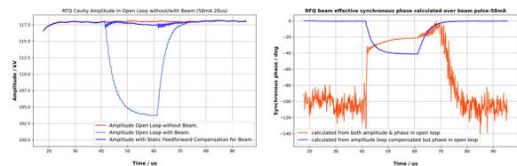
Figure 7: Uncompensated and compensated beam loading (left) and their effects on beam phase (right).
