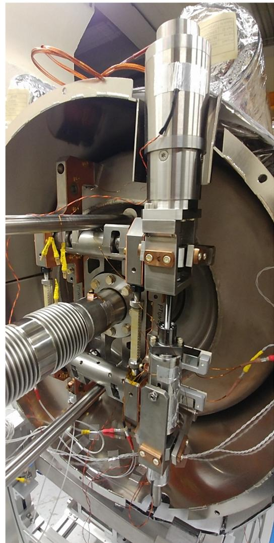
Figure 1: Prototype tuner assembled on a single-spoke cavity during cryomodule integration.
