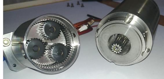
Figure 6: Gearhead (on the left) disassembled from the motor (on the right) after ALT.
