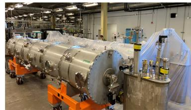
Figure 1: The first two cryomodules staged for installation in the front-end building.
