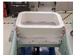
Figure 4: Taping of a chicane magnet winding (left) and the completed winding set (right).
