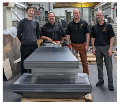
Figure 3: The first chicane magnet core at the vendor.
