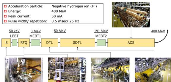
Figure 1: Configuration of J-PARC LINAC.
