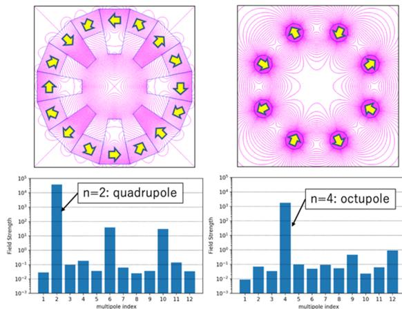
Figure 4: Produced quadrupole and octupole field in the prototype combined function magnet. The field was calculated with PANDIRA in Poisson/Superfish [9].
