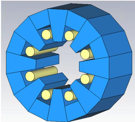
Figure 3: Designed configuration of permanent magnets for combined function focusing magnet.
