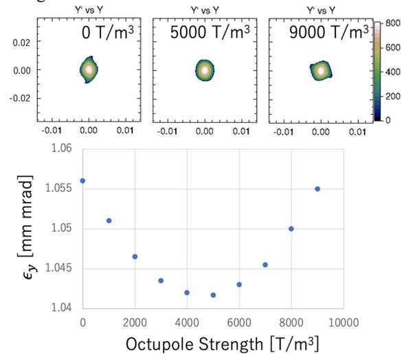
Figure 8: Results of the simulation. Upper figures show phase space distribution in vertical (y) axis of the extracted position. Lower figure shows the effect of octupole field strength on
