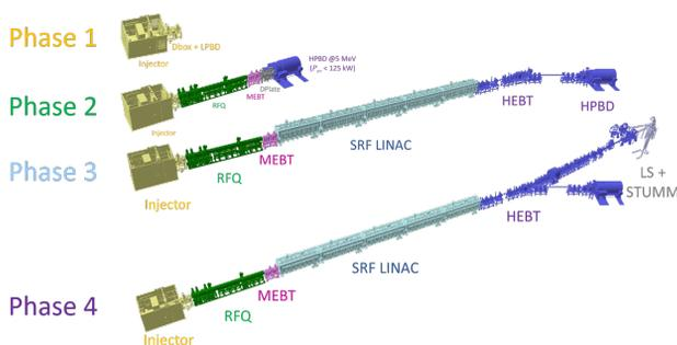
Figure 2: The accelerator during the different phases.
