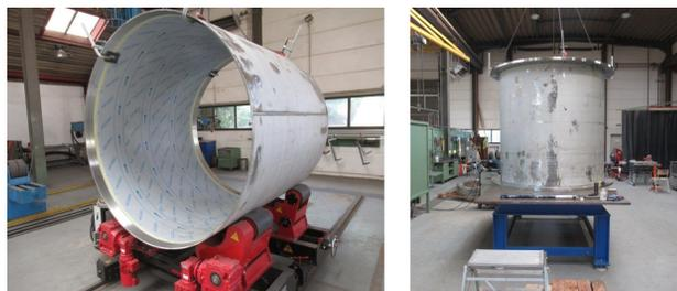
Figure 6: Rolling and welding of a cavity section.
