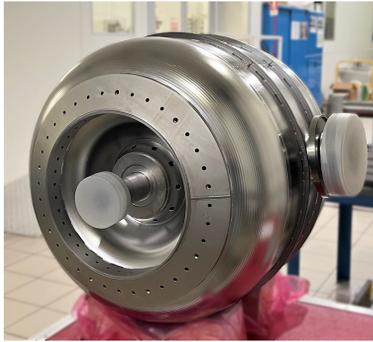
Figure 2: Pre-production SSR2 Bare Cavity.
