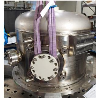
Figure 9: SSR2 Jacketed Cavity.
