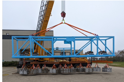
Figure 1: Transport frame 200% load test, or 30.4 tons.
