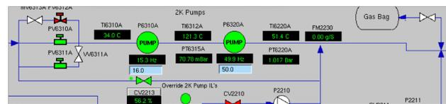
Figure 2: Bypass valve (CV2213) shown operating on PID control in parallel with 2 K main pump (P6320A) and booster pump (P6310A) (NB: direction of flow is left to right through pumps and right to left through bypass valve).
