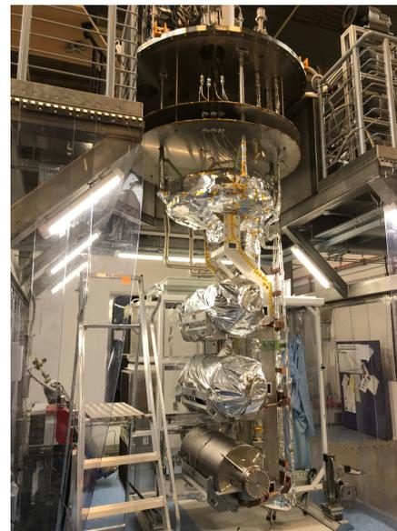
Figure 1: Photograph of CSI on stand with three jacketed cavities (top and middle cavities dressed in MLI jackets).
