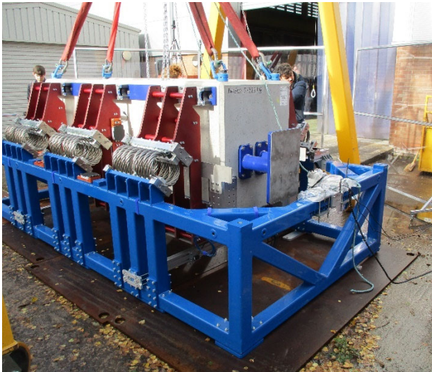
Figure 3: Drop test arrangement. Isolators between blue frame and red arms. Concrete mimics cryomodule mass.
