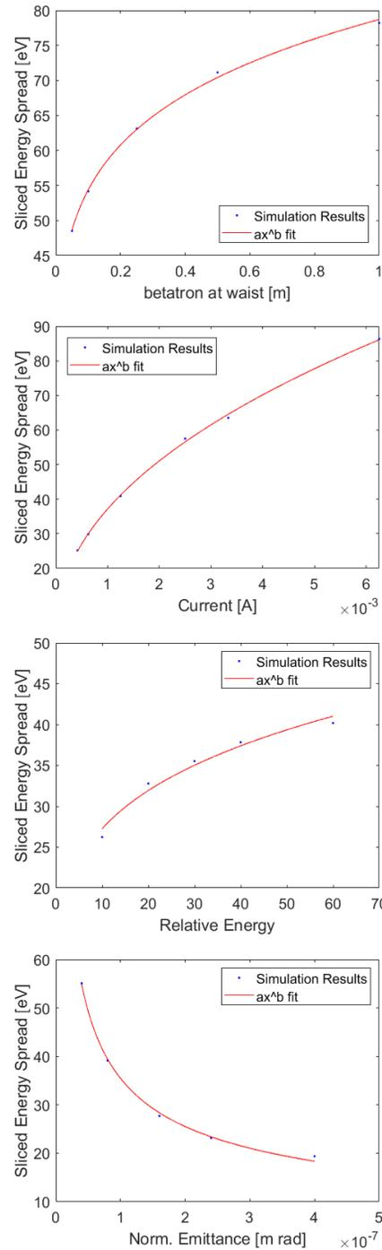
Figure 5: Parameter scan of certain beam parameters to find the dependence of sliced energy spread through a waist.
