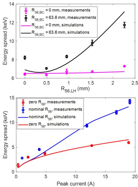
Figure 4: Sliced energy spread measurements in SwissFEL at the end of the injector for different bunch peak currents and compression levels in the bunch compressor [14].
