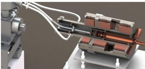
Figure 3: A rendering of the cryogenic S-band photogun [5].
