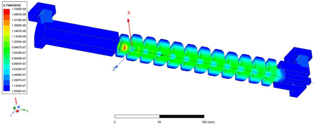
Figure 1: Electric fieldmap of the novel travelling-wave RF photogun.
