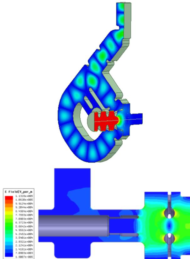
Figure 2: Two high gradient SW RF photogun projects which are underway investigating the idea of heavily overcoupled cavities [12, 13].
