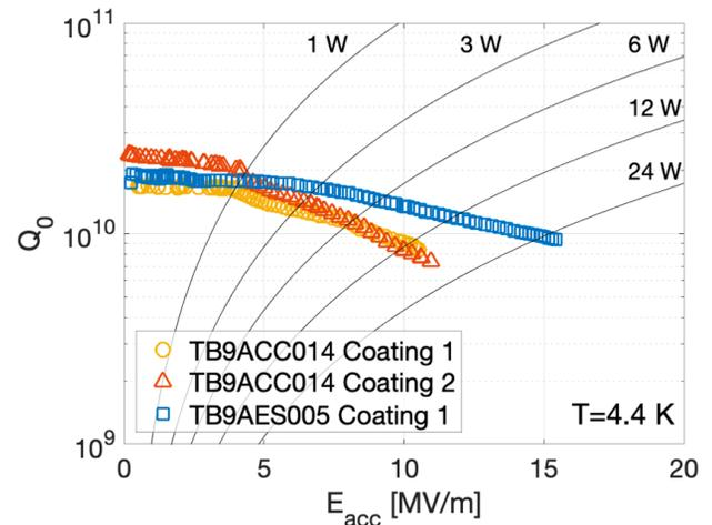
Figure 10: The Fermilab Nb<sub>3</sub>Sn 9-cell cavity RF data [7].
