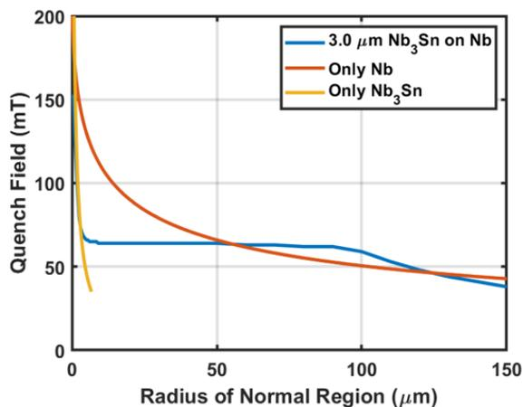
Figure 5: Thermal simulations showing how the Nb substrate is able to stabilize the Nb<sub>3</sub>Sn film allowing it to survive to higher fields before reaching cavity quench [1].
