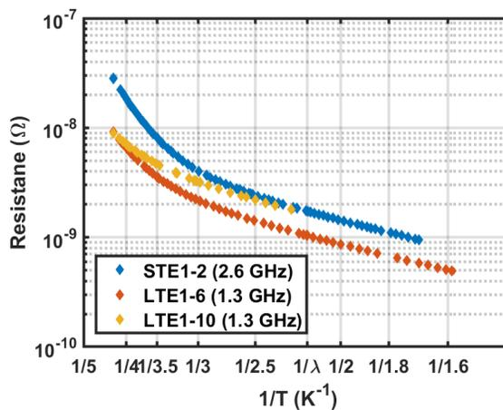
Figure 7: BCS resistance versus inverse temperature data for several typical Cornell ILC shaped Nb<sub>3</sub>Sn cavities of various frequencies [1].
