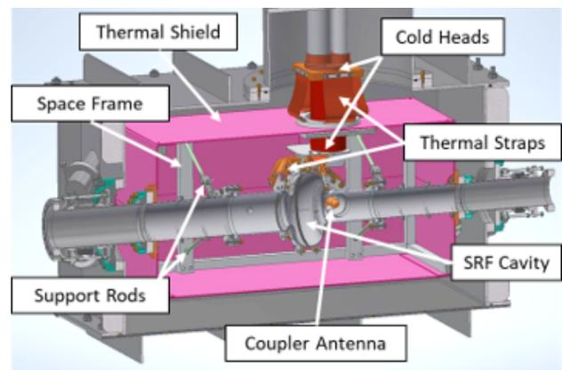
Figure 11: Schematic of the Cornell Compact Turn-Key Cryostat [17].
