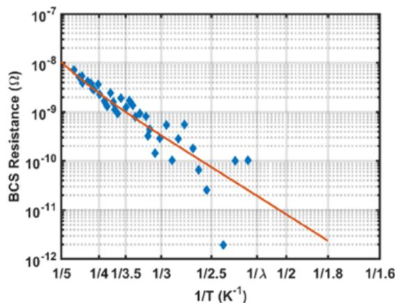
Figure 8: BCS resistance versus inverse temperature data for the Cornell thin film cavity which is a 1.3 GHz ILC shaped Nb<sub>3</sub>Sn cavity baked with higher Sn availability and a 1.5 μm thick film [1].
