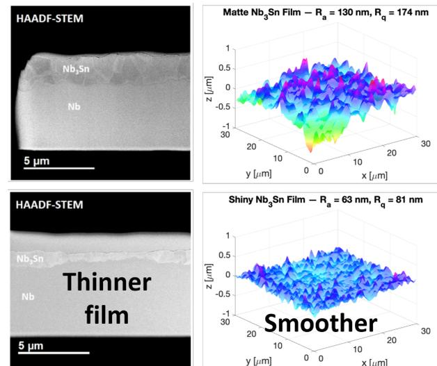
Figure 4: STEM images and 3D surface maps for the Fermilab thin and smooth coating [7].
