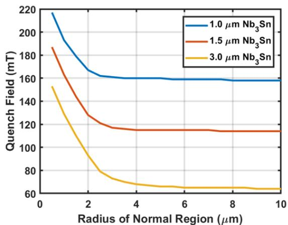
Figure 6: Simulation showing the maximum quench fields that can be supported at different thicknesses of Nb<sub>3</sub>Sn as a function of normal conducting region radius [1].
