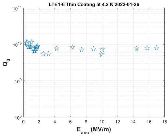
Figure 9: Q<sub>0</sub> versus E<sub>acc</sub> for the Cornell thin film cavity. Quench occurred at approximately 17 MV/m.
