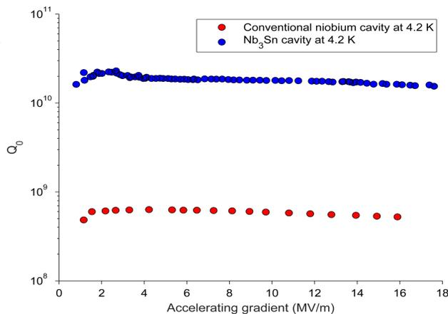
Figure 3: RF data comparing the early Nb<sub>3</sub>Sn work done at Cornell to Nb cavity RF data.
