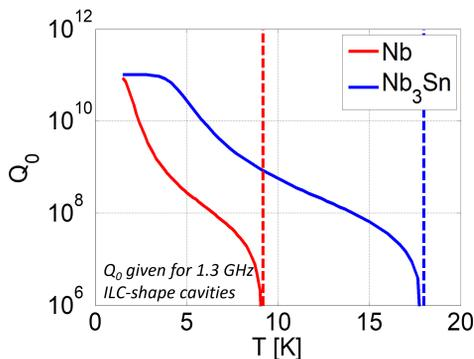
Figure 2:  $Q_0$  versus temperature. At 4.2 K, Nb<sub>3</sub>Sn significantly outperforms pure Nb. This figure shows that a 1.3 GHz Nb<sub>3</sub>Sn cavity could efficiently operate at 4.2 K rather than 2 K, which is the typical operation temperature for Nb cavities
