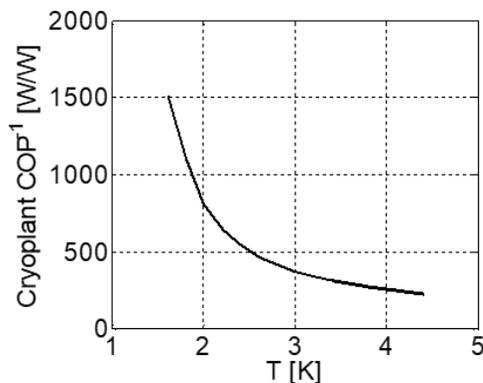
Figure 1: The cooling power, which is in watts of AC wall power needed to remove one watt of power from the cryogenic system, is much higher for low temperatures [2, 3].
