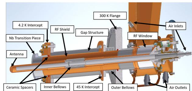
Figure 5: CAD model of the high-power input coupler for Cornell’s conduction-cooled cryomodule. Several key components are labeled on the figure.
