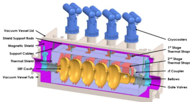
Figure 6: CAD model of the accelerating cryomodule used in Fermilab’s wastewater treatment design [15]. Some key components include 8 total cryocoolers (4 being visible), the 5-cell 650 MHz cavity, and the 4.2 K conduction path (visible above the cavity).
