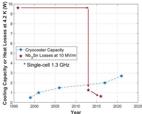
Figure 1: Progress in both Nb<sub>3</sub>Sn cavity performance (red stars) and pulse-tube cryocooler capacity at 4.2 K (blue curve) [10].
