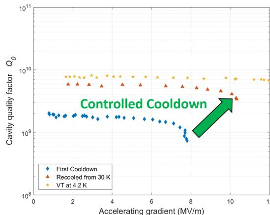
Figure 3: Example RF results from a proof-of-principle demonstration of operating a conduction-cooled Nb<sub>3</sub>Sn cavity at Cornell. The curve labeled “VT at 4.2 K” is from a vertical test in a helium bath and represents the baseline performance of this cavity, while the other two are from tests using the conduction cooling assembly. Note that the optimal performance was achieved after a more controlled cooldown, in this case achieved via temperature cycling the system.
