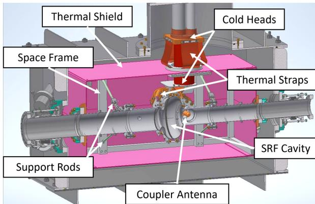
Figure 4: 3D model of the current design iteration of Cornell’s conduction cooled cryomodule. Some components of interest are labeled on the figure.
