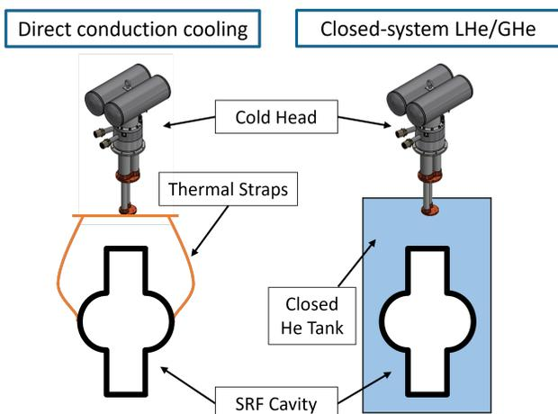
Figure 2: Two new cooling schemes which are possible using cryocoolers. Most cryomodule designs proposed today use the direct conduction cooling method.
