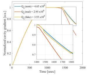
Figure 1: Normalized cavity gradient amplitude for a nominal, fake- and real-quenched pulse. The inset zooms on the decay section at the end of the pulse, when the RF is switched off.
