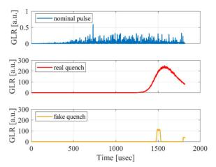
Figure 2: The Generalized Likelihood Ratio (GLR) proved to be a useful metric to categorize trips. The shape and magnitude of the GLRs differs greatly between trips.
