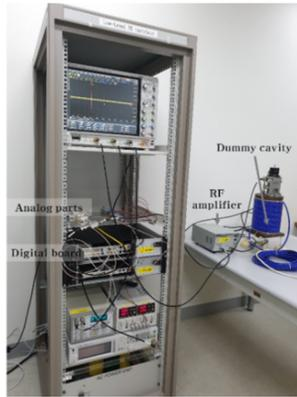
Figure 5: LLRF test stand setup.
