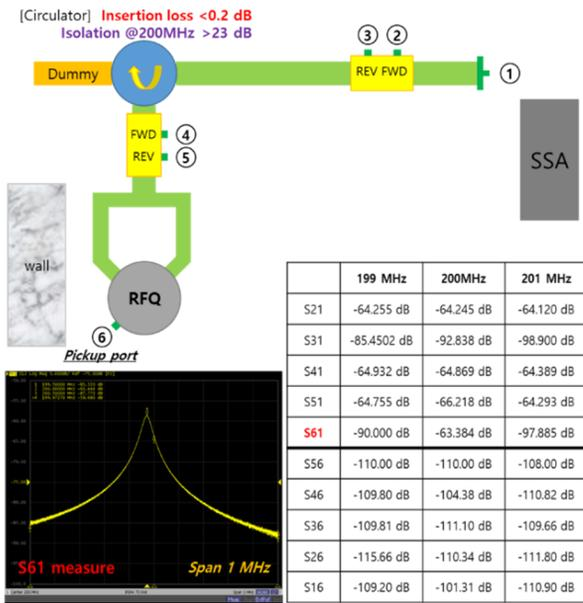
Figure 9: Measuring coupling coefficient.
