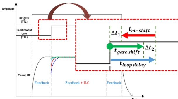
Figure 11: Time delay in the control loop.
