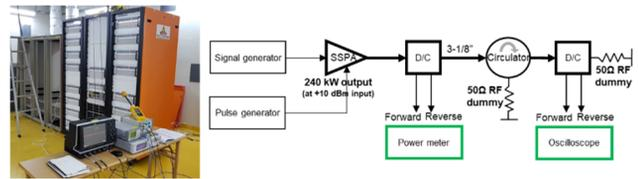
Figure 7: RF source driving test setup.
