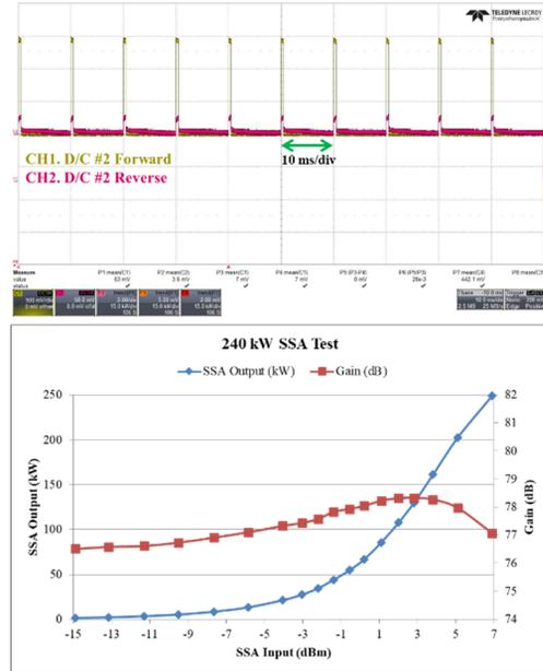
Figure 8: SSA test results.
