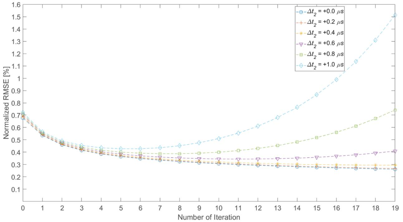
Figure A.1: Results of the simulation study on time delay effect on ILC.
