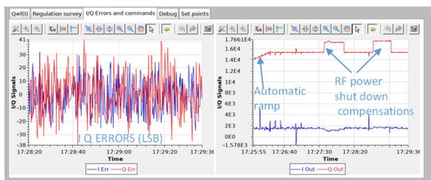
Figure 6: IQ errors and drive during a ramp and PSSA modules shut down.
