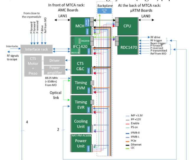
Figure 2: MTCA based LLRF prototype system scheme.
