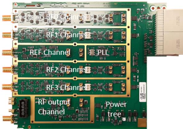
Figure 3: RFC1470  $\mu$ RTM prototype board (IOXOS Technologies).
