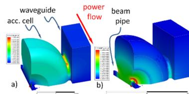
Figure 1: Quarter-cell finite element model of the  $\beta = 1$ , 9.3 GHz, 120 deg. phase advance per cell traveling wave accelerating
