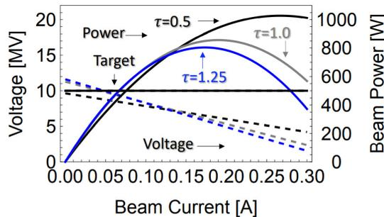
Figure 2: The net voltage gain and average beam power for the constant gradient structure with length of 60 cm. Solid curves show average beam power for magnetron duty factor of 0.08%. Dashed curves show beam loaded output energy. It can be seen from the graph that the linac with attenuation factor  $\tau = 1$  is the closest to achieving the target parameters, and the result is not sensitive to the small change of  $\tau$ . For details, see [4].
