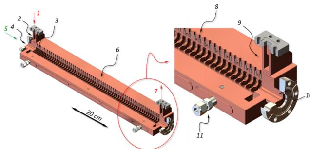
Figure 5: Solid model of a high efficiency traveling wave accelerating structure. Upper left part is cut to show internal geometry. This is a 9.3 GHz,  $2\pi/3$  phase advance structure. Notation as follows: 1 – input RF power; 2 – input waveguide; 3 – low  $\beta$  section for beam bunching; 4 – input
