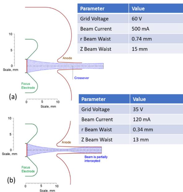
Figure 4: Results of beam dynamics simulations of 30 kV triode gun.
