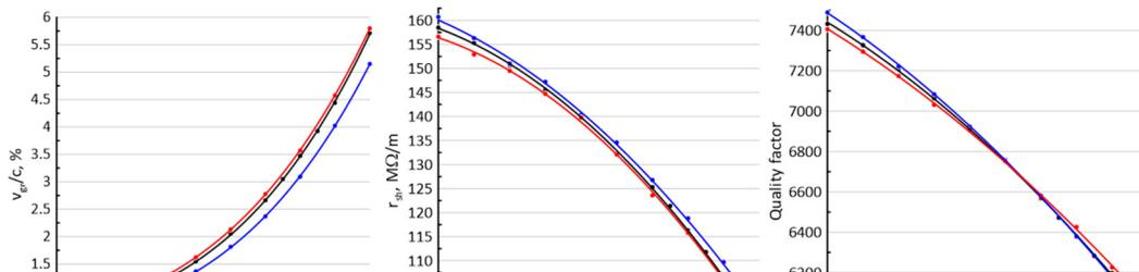
Figure 3: Group velocity (a), shunt impedance (b), and  $Q_0$  vs transverse hole's size,  $h_y$  for longitudinal sizes  $h_z$ : 5 mm (blue), 6 mm (black), and 7 mm (red). The structure is 9.3 GHz, traveling wave with 120 deg. phase advance per cell.
