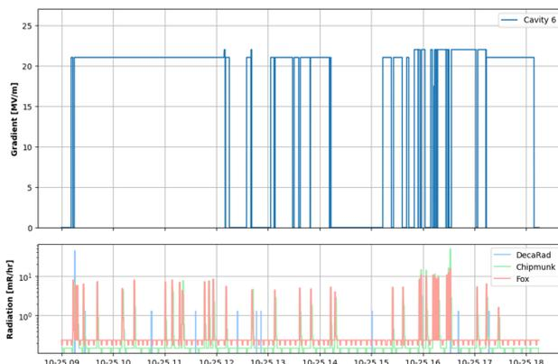
Figure 2: MP Processing – Cavity gradient (above) and radiation (below). Here one can see a quench followed by a stable run for approximately 2hr before repetitive quenching and processing.
