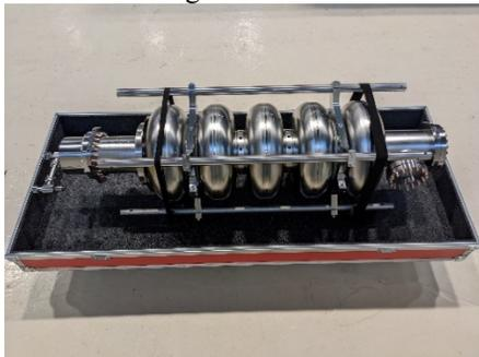
Figure 6: HB03 ESS-prototype cavity ( $\beta=0.86$ ) to be treated by VEP with dedicated cathode after RF test.
