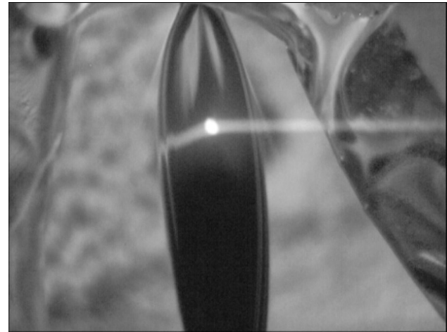
Figure 4: Lithium film jet receiving 300-W ( 65 \text{ MW/cm}^3 ) 65-keV CW proton beam [7]
