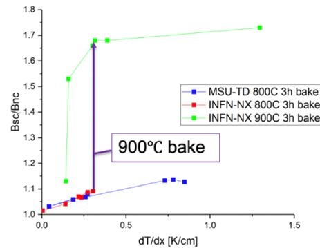
Figure 4: Measured single cell cavity flux expulsion as a function of the spatial temperature gradient along the cell surface.
