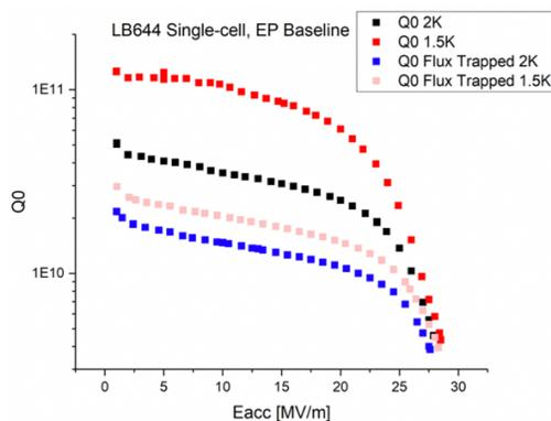
Figure 3: Flux sensitivity measurement in an electropolished single-cell FRIB400 cavity.
