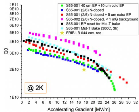
Figure 2: Cold tests at 2 K for the FRIB400 prototype cavities (S65-001, -002) before and after N-doping or FMTB. The yellow star marks the FRIB400 minimum goal.
