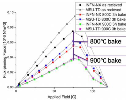
Figure 5: Flux-pinning force as a function of applied magnetic field measured on Nb samples using the PPMS.
